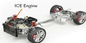
Image 1 - Chassis platform for an Internal Combustion Engine (ICE) vehicle
